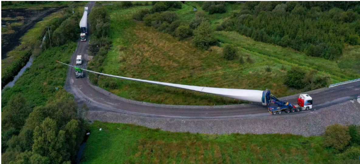
[Collett of Halifax delivery of 80-metre blade showing ability to oversail corners. The rear is on an independent dolly, and 10-metres of blade end can also oversail.]
