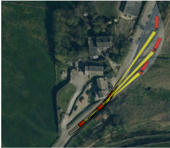
Bank excavation to pass Dale View Farm: WTRG
