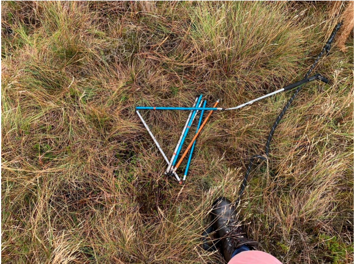
The 3-metre avalanche pole broke as it was extracted from full depth at Crow Hill Junction. It died doing what it loved. WTRG
